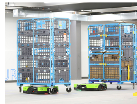
Fig. 1: Amazon’s Proteus robots [1] carry uniform loads and are example platforms that can be used for multi-robot ordered storage and retrieval in warehouses.
