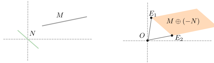
Fig. 5: Left: Two segments M and N , where M is fixed. Right: Configuration space Q(N) and Minkowski difference between M and N .
