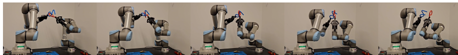
Fig. 6: Execution of a CMG-RRT planned trajectory for the az puzzle using two UR5e robotic arms. Arms trajectories are based on a separate continuous IK derived from the exact CMG-RRT trajectory for the free-flying objects.
