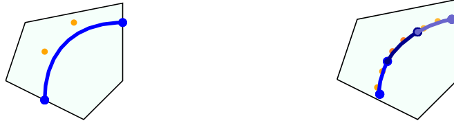
(a) The shortest-path formulation from [38] optimizes a Bézier curve and its duration, resulting in non-convex acceleration constraints. (b) Our shortest-walk formulation searches for a fixed-duration Bézier curve per vertex visit, resulting in convex acceleration constraints.
